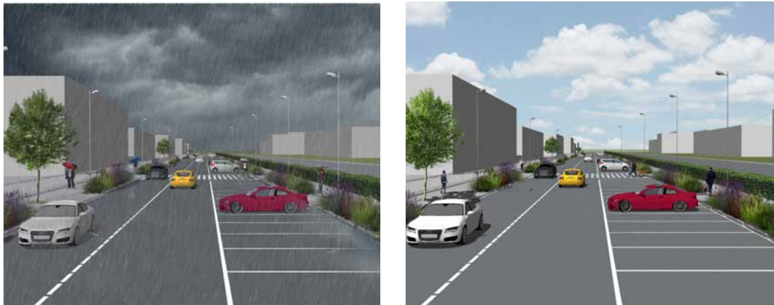
Figure 3. Rendering of the chosen solution (Alternative 3, bioretention areas) in the project scenario, in rainy weather (left) and dry weather (right)
